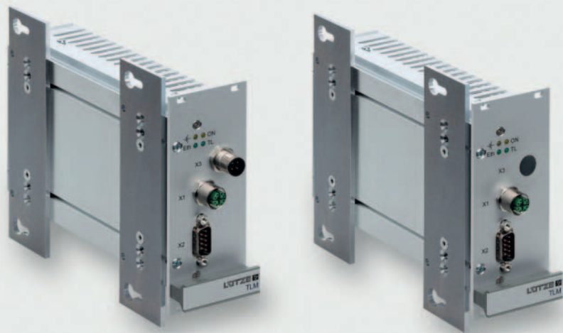
Train Line Modems TLM-X and TLM-10 enable gigabit Ethernet across existing lines throughout the train via the coupling
